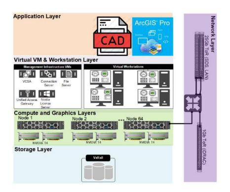
VDI Solution Stack with Esri ArcGIS Pro and Engineering CAD software
